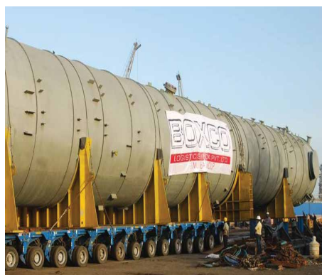
The 91m long C2 splitter at Mumbai port using SPMTs
